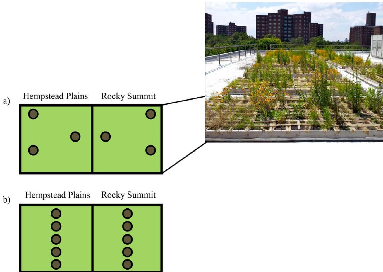
**Figure 2. Sampling scheme for the general (a) and fine-scale (b) sampling with an image of a representative green roof.** The general sampling scheme was used for all ten green roofs and the six cores were composited for three planting boxes on each roof. For the fine-scale sampling on the three target roofs, each core was treated as a separate sample. doi:10.1371/journal.pone.0058020.g002
